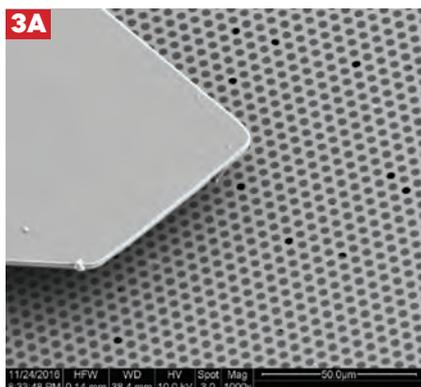
**FIGURE 3A**, above, The SEM screens a series of single and double layer graphene membranes. The AFM tip is then positioned at the region of interest to probe a specified area of interest further at higher resolution
