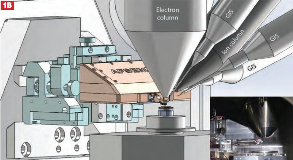
**FIGURE 1A**, top, AFSEM™ module that fits directly into the SEM chamber
