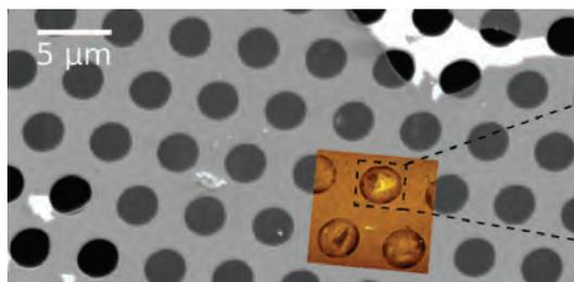
**FIGURE 3B**, above, An array of unsupported single and double layer graphene membranes visible with the SEM. The AFM has imaged an area covering several of these membranes in the orange square and provide high-resolution 3D info as shown in the zoomed in image on the right of one of the membranes displaying the sub-nanometer resolution capability
